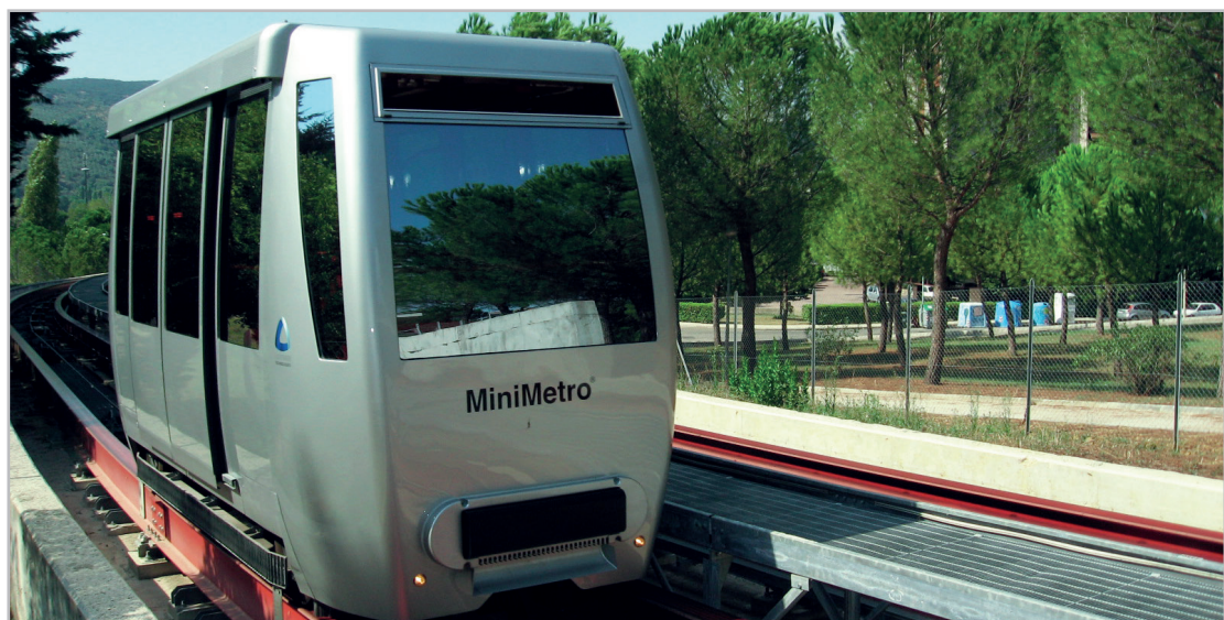
Figure 12: MiniMetro Perugia, urban detachable funicular system (TÜV SÜD Industrie Service GmbH)
