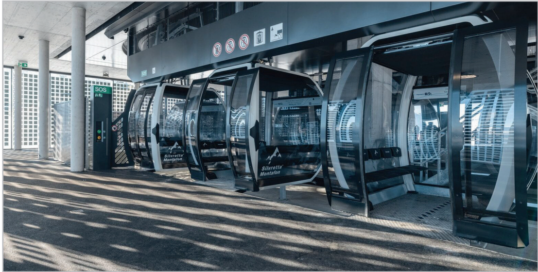
Figure 14: Autonomous operating ropeway with special infrastructure (Doppelmayr, 2024a)
