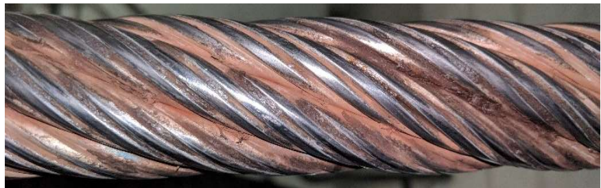
Corrosion induced by friction between touching strands
