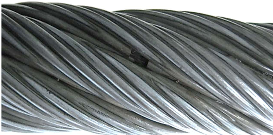
Common wire break due to bending cycles
