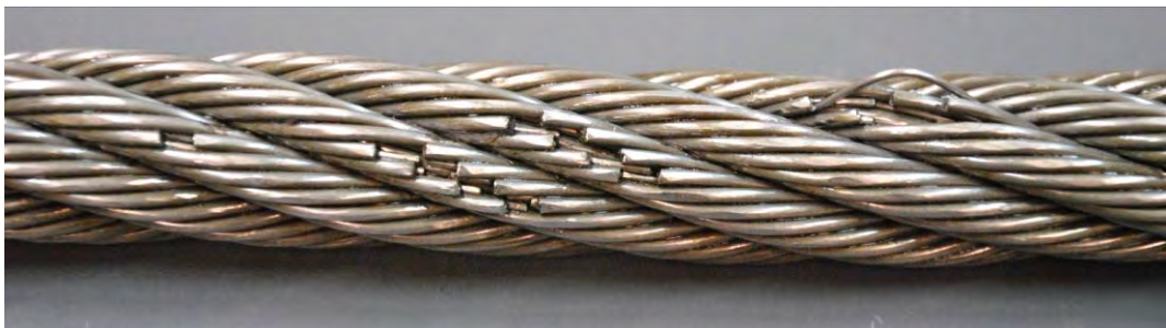
100% bending cycles zone (close to failure)
