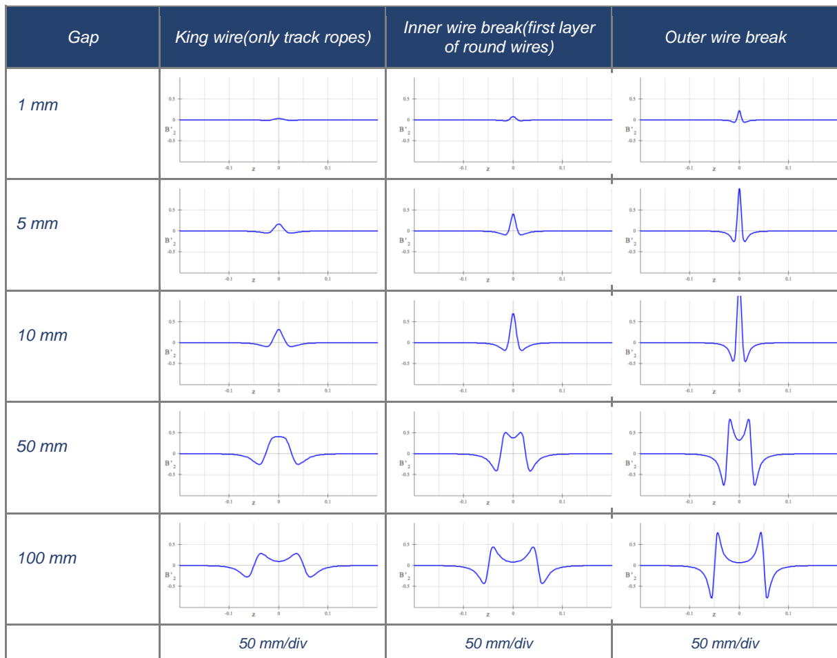
Figure 25: Different search patterns as a function of the distance between the fracture faces of a wire (gap) and the position of the wire within the rope.
