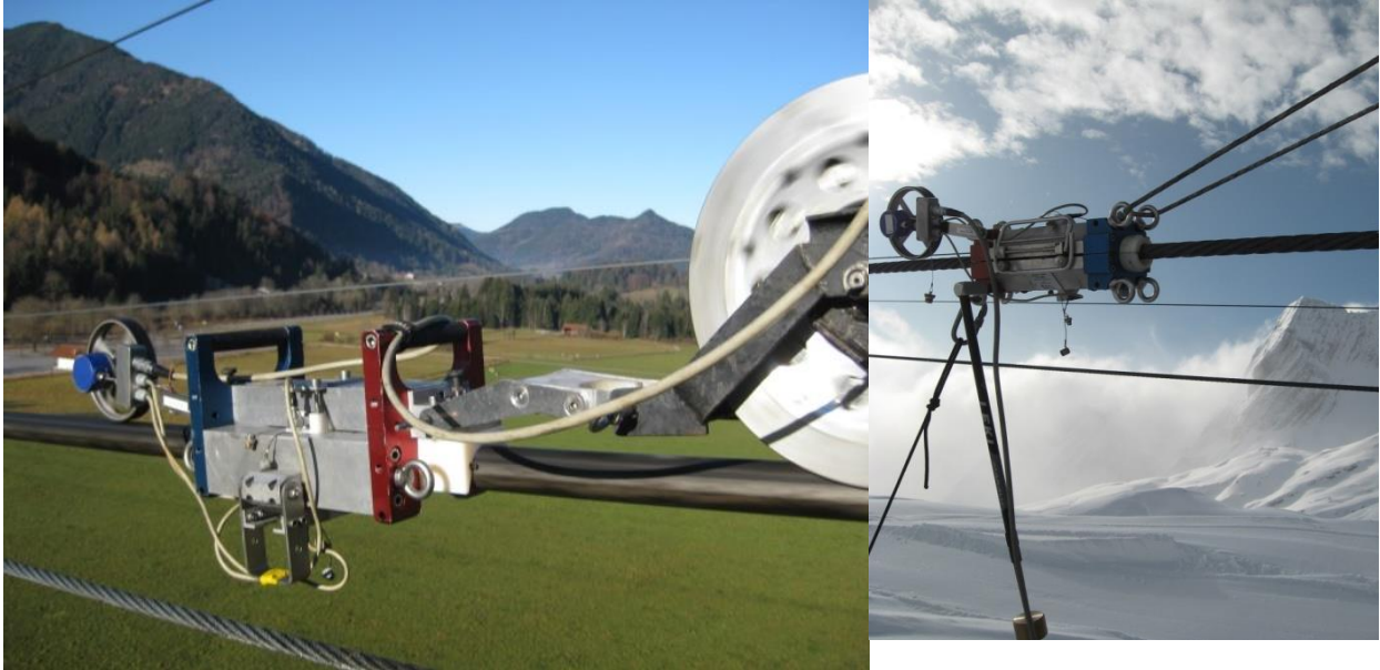
Figure 22: Set-up of MRT device on a fixed rope (left), and moving rope (right).
