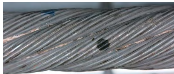
Figure 4-14: Wire break 0.5 x strand diameter
