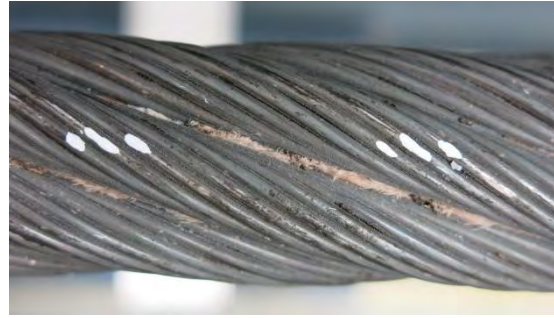
Figure 4-28: Artificial hair lines/ notches
