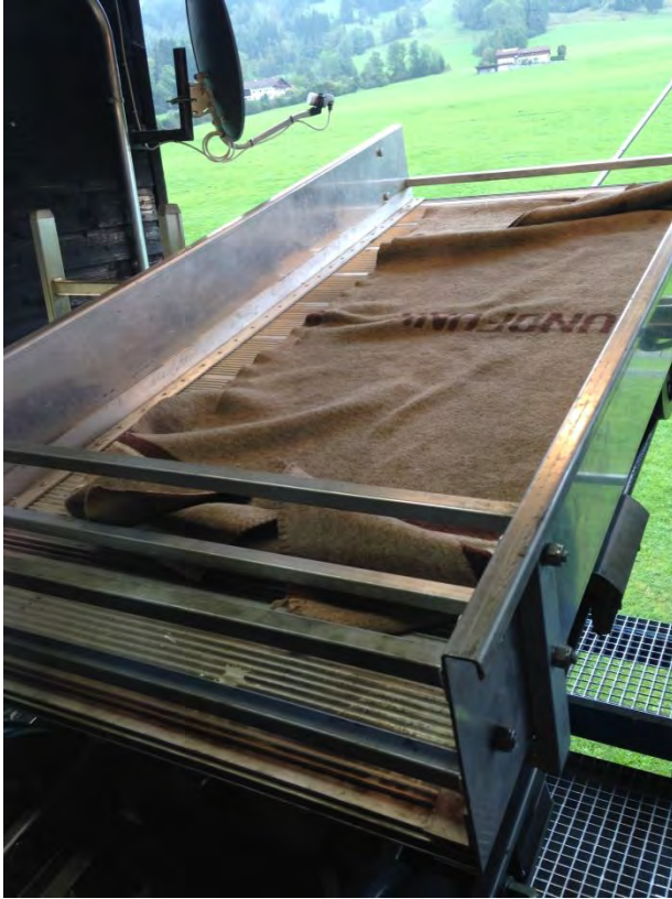
Figure 5-27: Platform to lie down during visual inspection
