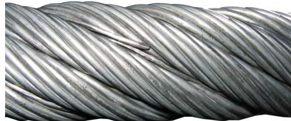
Figure 4-9: Wire break with protruding wire
