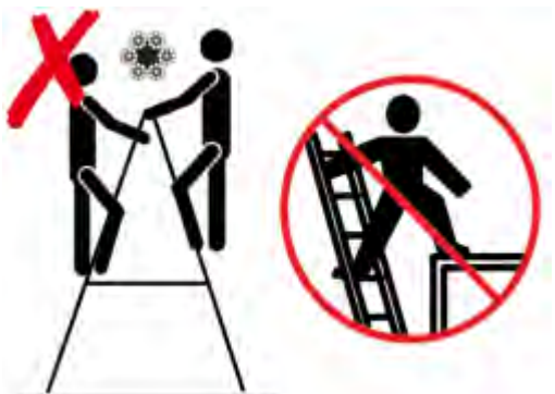
Picture 9: Not recommended usage of ladders
