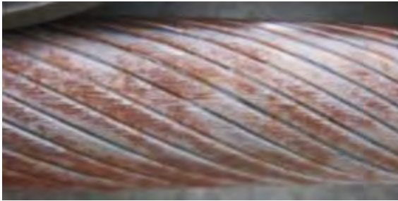
Locked coil rope – hair lines / notches
