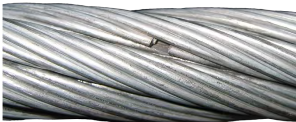
Figure 4-8: Single wire break
