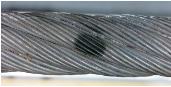
Figure 4-15: Wire break 1.0 x strand diameter
