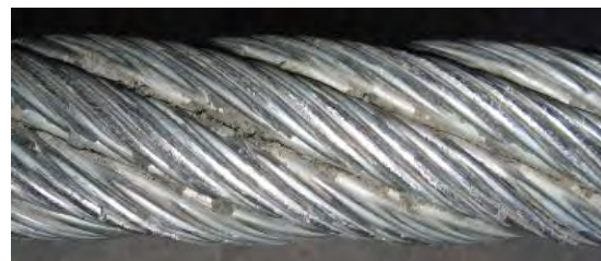
Figure 4-26: Hair lines on a hauling rope
