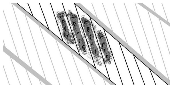
Figure 4-20: Corrosion on several strands abstracted
