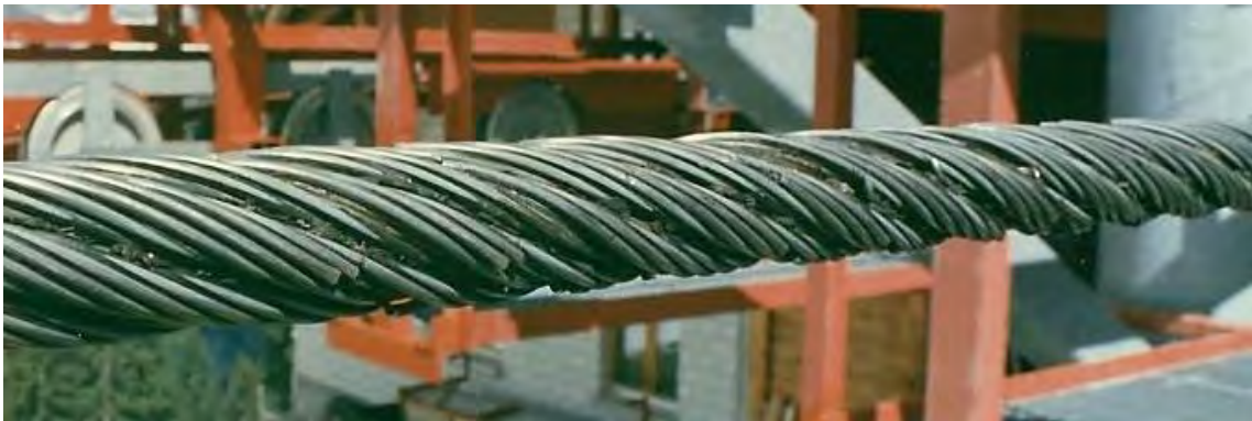
Figure 2-1: Damages of slipped mounting clamp
