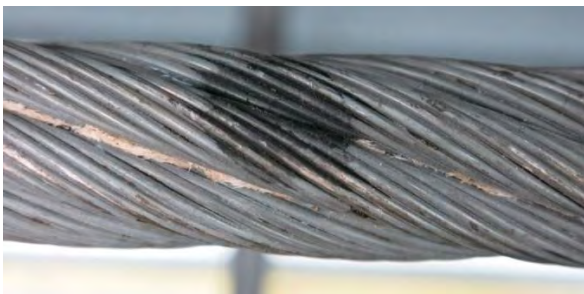
Figure 4-4: Lightning strike 1.5 x strand diameter
