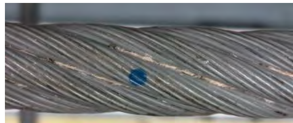
Figure 4-7: Lightning strike 0.5 x strand diameter
