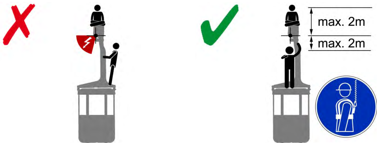
Picture 11: Bad position during track rope inspection. About 45 ° of the rope aren't visible
