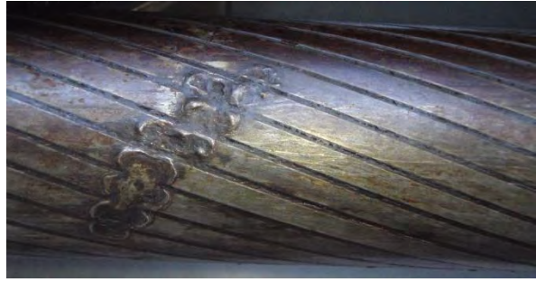
Figure 2-15: Point of escape at the side of the rope
