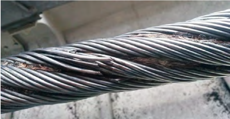
Figure 2-3: Shrunken tuck tail ends with several wire breaks
