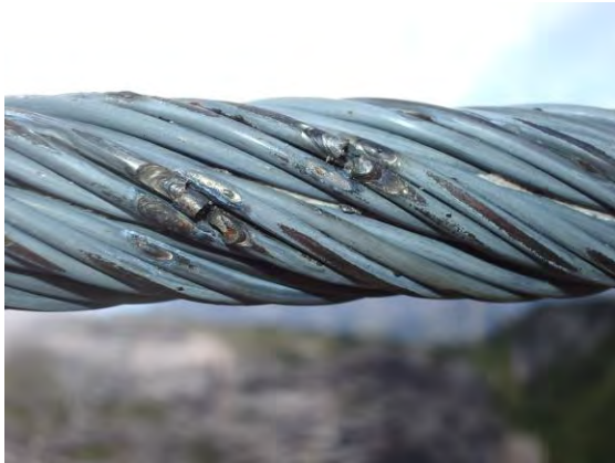
Figure 4-2: Martensite with molten wires
