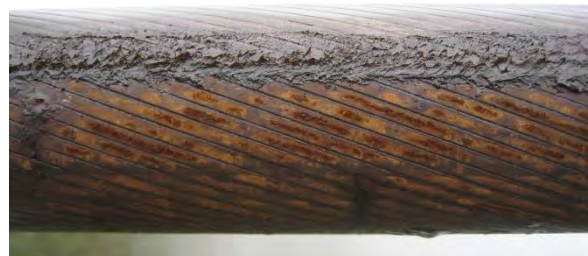
Figure 4-18: Corrosion at fully locked coil rope
