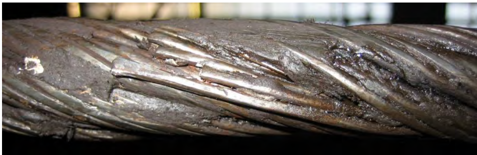
Figure 6-13: Dirty rope - inspection not possible
