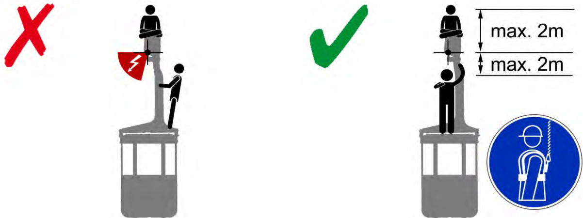
Figure 6-11: Bad position during track rope inspection. About 45 ° of the rope are not visible
