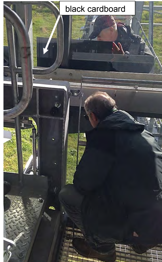
Figure 5-24: Applying black cardboard as sun protection
