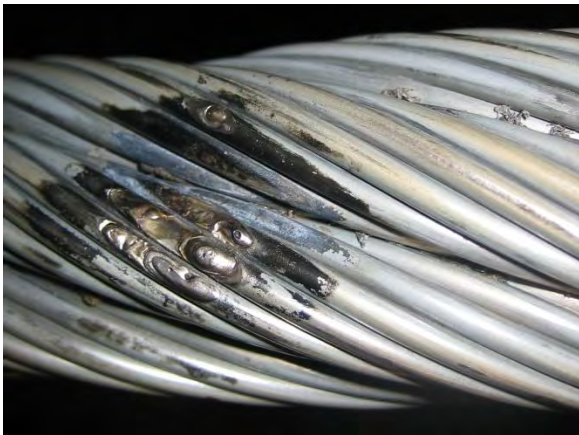
Figure 2-10: Lightning strike at strand rope
