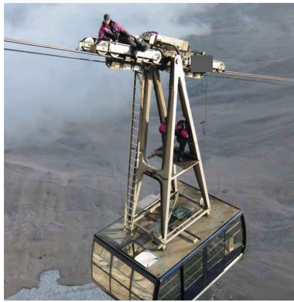
Figure 3-9: Visual inspection of track ropes on a platform and the carrier truck
