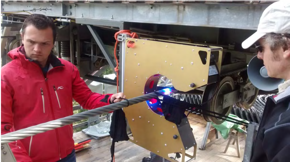
Figure 5-18: Inspection with nylon stocking
