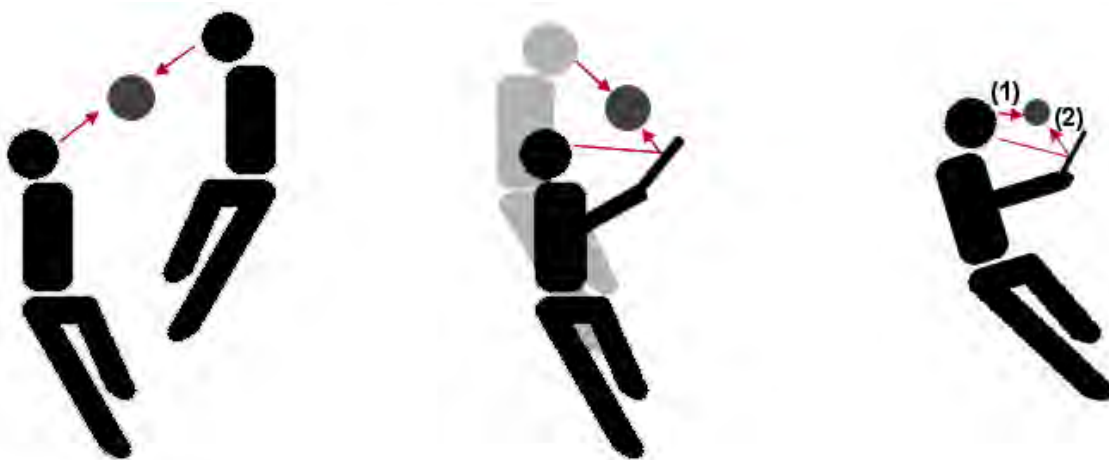
Figure 3-7: Possible viewing directions of inspectors during an inspection
