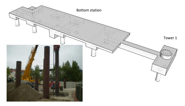
Having taken this into account the station's foundation was built with Pile driving steel tubular – 8 units with 30m deep.
