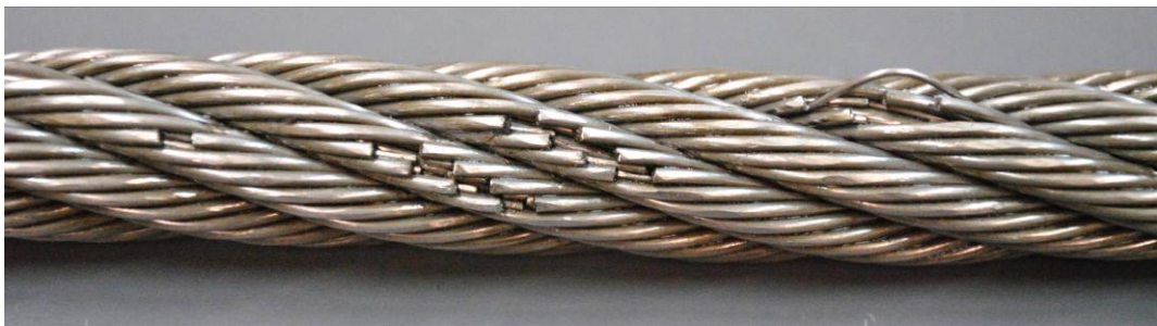
100% bending cycles zone (close to failure)
