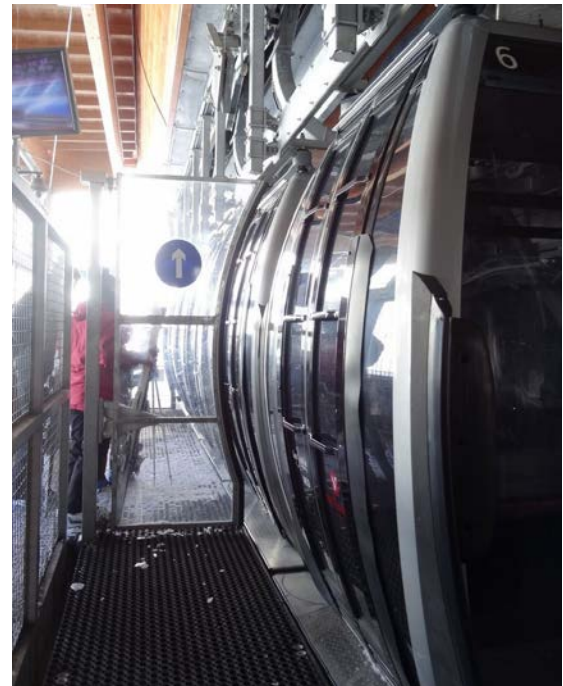
Another solution was used for continuous movement gondola Cairn-Caron (still in Val Thorens), with a “moving cabin wall” in unmanned stations. There are some specific parts added on the cabin sides so as to prevent a fall between cabins. Some chain claws up in the station tracks allow to manage the space between cabins, and guides are added in the upper part to for a good equilibration of the cabin. Physical screens prevent people from going further outside cabins ; sensible platforms have also been put next to these screens so as to stop the installation in case of a bad loading/unloading.
