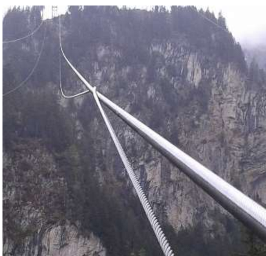
Rollover of a hauling rope
