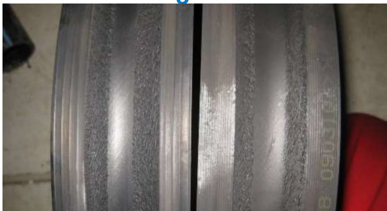
Small lining grooves lead to wear at the edges and to twisting
