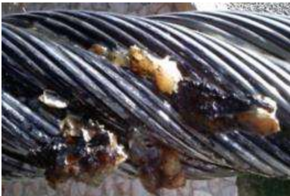
Heat impact on a carrying-hauling rope
