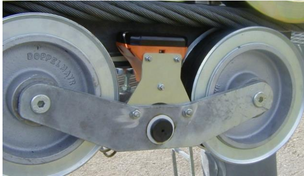
RPD – Rope Position Detection since 1997
