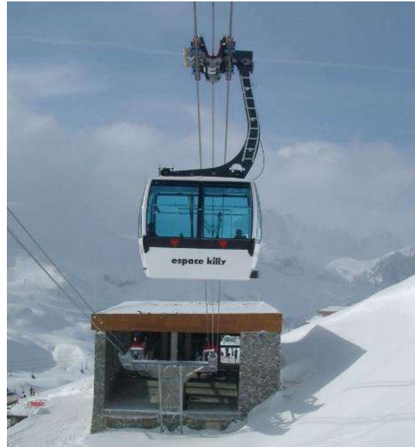
2002 L'Olympique in Val d'Isère is the first tri-cable gondola lift built by Doppelmayr.
