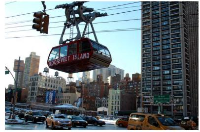
Tram, it was ultimately decided to replace the Tram rather than to remove it. As part of the USD25 million renovation, the system was reconfigured to be two parallel independent single reversible trams (or a dual haul system) using the original tower and station infrastructure. The new system opened in November 2010. Today the tram carries more than 2.5 million passengers annually between Roosevelt Island and Manhattan.
