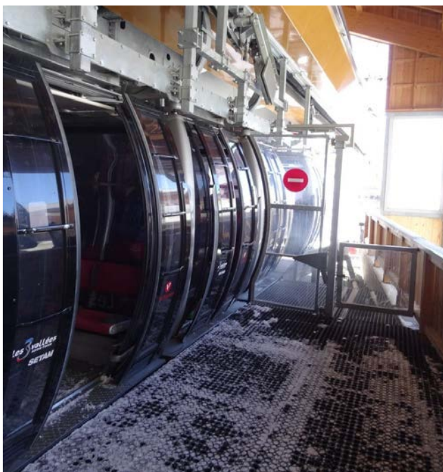
Another solution was used for continuous movement gondola Cairn-Caron (still in Val Thorens), with a “moving cabin wall” in unmanned stations. There are some specific parts added on the cabin sides so as to prevent a fall between cabins. Some chain claws up in the station tracks allow to manage the space between cabins, and guides are added in the upper part to for a good equilibration of the cabin. Physical screens prevent people from going further outside cabins ; sensible platforms have also been put next to these screens so as to stop the installation in case of a bad loading/unloading.
