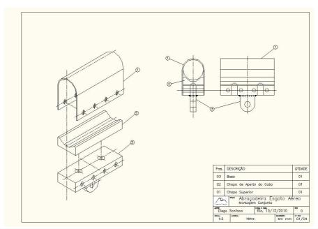
Schematic - Assembly of Top Clamp
