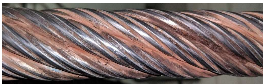
Corrosion induced by friction between touching strands
