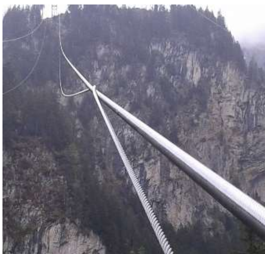
Rollover of a hauling rope
