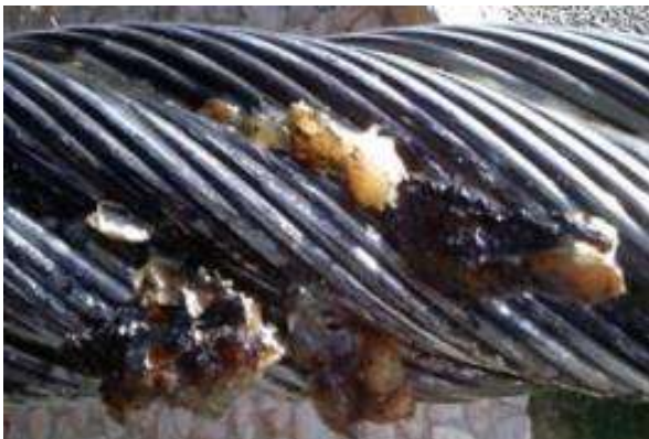
Heat impact on a carrying-hauling rope
